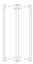
insert each bulb parallel (90°) to the Eiffel frame
